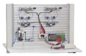
The Basic Electro-Pneumatic trainer kit is designed with capability to demonstrate the design, construction and application of Electro pneumatic components and circuits. Applicable to various disciplines in academic institutions like Mechanical, Mechatronics, Production, Instrumentation and more, and for companies having ISO & TPM training systems.
